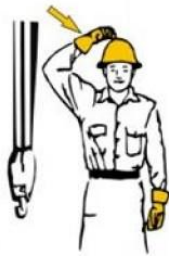
Use Main Hoist
